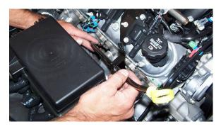
Remove the spark plug wires from both the coil packs and the spark plugs on both engine banks.
