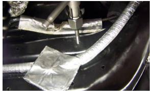
Install the clamp so that the curved part cradles the clutch line and clamps it loosely to the firewall.
