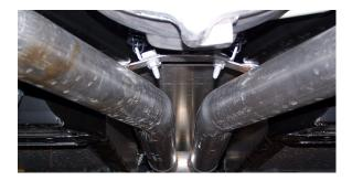
• After completing the removal of the cross brace bracket nuts, move forward in the vehicle and remove the four (4) nuts holding the tail pipe assembly to the down tubes. Be careful to support the front end of the tail pipe assembly as the last of the nuts is removed. You may need some help at this point to slip the tail pipe assembly off of the muffler inlet tubes. It is best to do one side at a time until both are removed. The assembly can then be removed from beneath the vehicle.
