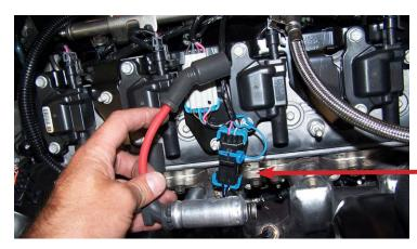
Front 02 sensor connector on the left (driver) side.
