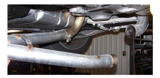
• The next step is to loosen and the remove the down tube/catalytic converter from the cast manifold on the left (driver) side.
